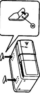
**2** Remove any dirt or stains from the surface you're going to mount the unit on, then attach the unit.
