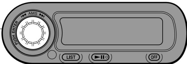
On this unit, listen to MD with an FM tuner. Therefore, if there is an FM broadcast with the same frequency as the frequency set on this unit (transmitted from this unit to the FM tuner), noise may occur during MD playback. In that case, change the transmission frequency of this unit. The initial value is 88.3MHz.
