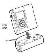
When the battery is completely charged, the CHG lamp goes off.
