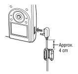
**3** Close the ferrite core. Make sure the clasps are fully engaged.
